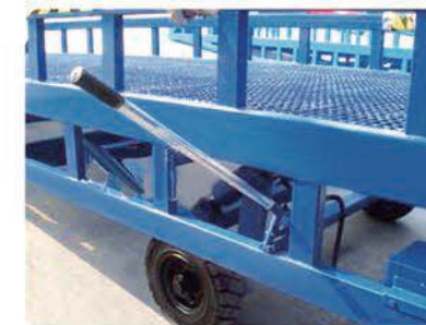
Manual hydraulic pump no need electric
